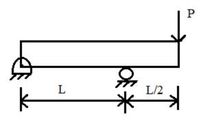
4. A continuous beam of uniform cross-section supported and loaded as shown in Figure. Draw the shear force and bending moment diagrams if the supports B and C sink by 25 mm and 10 mm respectively.
